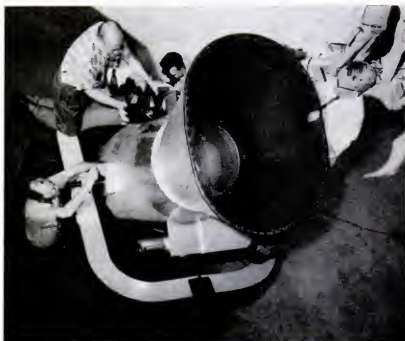
GIANT CAMERA photographs satellite against background of stars, for highest-precision tracking. Here is the first picture it caught of Sput-
